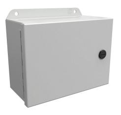
Hammond Eclipse Junior series enclosure, NEMA 3R/4/12/13, 6 x 8 x 3in (HxWxD), wall mount, carbon steel, RAL 7035 light gray, powder coat finish, single-door, 1/4-turn semi-flush latch.
