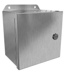
Hammond Eclipse Junior series enclosure, NEMA 3R/4/4X/12/13, 6 x 6 x 4in (HxWxD), wall mount, 316 stainless steel, #4 brush finish, single-door, 1/4-turn semi-flush 316 stainless steel latch.
