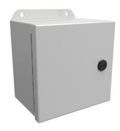
Hammond Eclipse Junior series enclosure, NEMA 3R/4/12/13, 6 x 6 x 4in (HxWxD), wall mount, carbon steel, RAL 7035 light gray, powder coat finish, single-door, 1/4-turn semi-flush latch.
