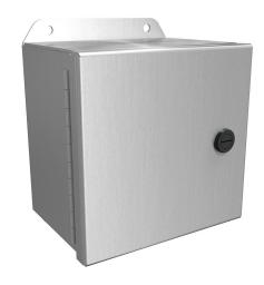
Hammond Eclipse Junior series enclosure, NEMA 3R/4/4X/12/13, 6 x 6 x 4in (HxWxD), wall mount, 5052-H32 aluminum, singledoor, 1/4-turn semi-flush 316 stainless steel latch.
