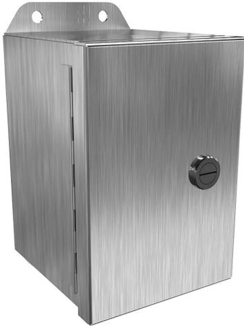
Hammond Eclipse Junior series enclosure, NEMA 3R/4/4X/12/13, 6 x 4 x 4in (HxWxD), wall mount, 304 stainless steel, #4 brush finish, single-door, 1/4-turn semi-flush 316 stainless steel latch.
