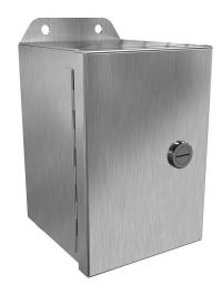
Hammond Eclipse Junior series enclosure, NEMA 3R/4/4X/12/13, 6 x 4 x 4in (HxWxD), wall mount, 316 stainless steel, #4 brush finish, single-door, 1/4-turn semi-flush 316 stainless steel latch.
