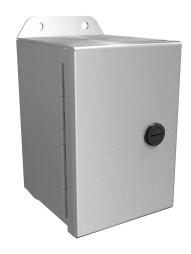
Hammond Eclipse Junior series enclosure, NEMA 3R/4/4X/12/13, 6 x 4 x 4in (HxWxD), wall mount, 5052-H32 aluminum, singledoor, 1/4-turn semi-flush 316 stainless steel latch.
