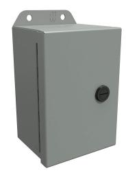
Hammond Eclipse Junior series enclosure, NEMA 3R/4/12/13, 6 x 4 x 3in (HxWxD), wall mount, carbon steel, ANSI 61 gray, powder coat finish, single-door, 1/4-turn semi-flush latch.
