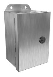
Hammond Eclipse Junior series enclosure, NEMA 3R/4/4X/12/13,  $6 \times 4 \times 3$  in (HxWxD), wall mount, 304 stainless steel, #4 brush finish, single-door, 1/4-turn semi-flush 316 stainless steel latch.
