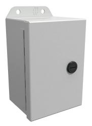
Hammond Eclipse Junior series enclosure, NEMA 3R/4/12/13, 6 x 4 x 3in (HxWxD), wall mount, carbon steel, RAL 7035 light gray, powder coat finish, single-door, 1/4-turn semi-flush latch.
