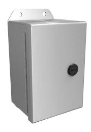
Hammond Eclipse Junior series enclosure, NEMA 3R/4/4X/12/13, 6 x 4 x 3in (HxWxD), wall mount, 5052-H32 aluminum, singledoor, 1/4-turn semi-flush 316 stainless steel latch.
