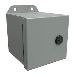
Hammond Eclipse Junior series enclosure, NEMA 3R/4/12/13, 4 x 4 x 4in (HxWxD), wall mount, carbon steel, ANSI 61 gray, powder coat finish, single-door, 1/4-turn semi-flush latch.
