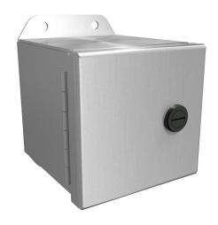
Hammond Eclipse Junior series enclosure, NEMA 3R/4/4X/12/13, 4 x 4 x 4in (HxWxD), wall mount, 5052-H32 aluminum, singledoor, 1/4-turn semi-flush 316 stainless steel latch.
