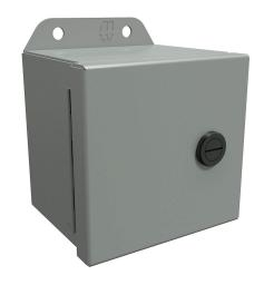
Hammond Eclipse Junior series enclosure, NEMA 3R/4/12/13,  $4 \times 4 \times 3$  in (HxWxD), wall mount, carbon steel, ANSI 61 gray, powder coat finish, single-door, 1/4-turn semi-flush latch.
