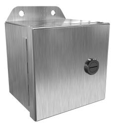
Hammond Eclipse Junior series enclosure, NEMA 3R/4/4X/12/13,  $4 \times 4 \times 3in$  (HxWxD), wall mount, 304 stainless steel, #4 brush finish, single-door, 1/4-turn semi-flush 316 stainless steel latch.
