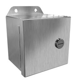
Hammond Eclipse Junior series enclosure, NEMA 3R/4/4X/12/13,  $4 \times 4 \times 3$  in (HxWxD), wall mount, 316 stainless steel, #4 brush finish, single-door, 1/4-turn semi-flush 316 stainless steel latch.
