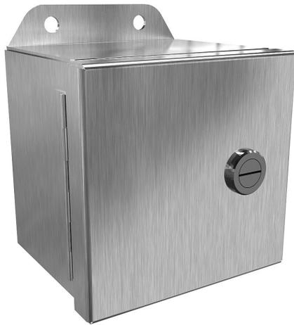
Hammond Eclipse Junior series enclosure, NEMA 3R/4/4X/12/13, 4 x 4 x 3in (HxWxD), wall mount, 316 stainless steel, #4 brush finish, single-door, 1/4-turn semi-flush 316 stainless steel latch.
