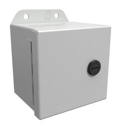
Hammond Eclipse Junior series enclosure, NEMA 3R/4/12/13, 4 x 4 x 3in (HxWxD), wall mount, carbon steel, RAL 7035 light gray, powder coat finish, single-door, 1/4-turn semi-flush latch.
