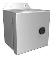
Hammond Eclipse Junior series enclosure, NEMA 3R/4/4X/12/13,  $4 \times 4 \times 3in$  (HxWxD), wall mount, 5052-H32 aluminum, single-door, 1/4-turn semi-flush 316 stainless steel latch.
