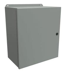
Hammond Eclipse Junior series enclosure, NEMA 3R/4/12/13, 16 x 14 x 8in (HxWxD), wall mount, carbon steel, ANSI 61 gray, powder coat finish, single-door, 1/4-turn semi-flush latch.
