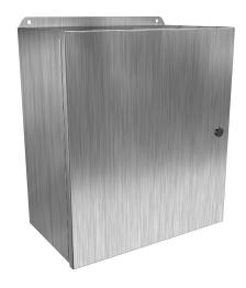
Hammond Eclipse Junior series enclosure, NEMA 3R/4/4X/12/13, 16 x 14 x 8in (HxWxD), wall mount, 304 stainless steel, #4 brush finish, single-door, 1/4-turn semi-flush 316 stainless steel latch.
