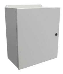
Hammond Eclipse Junior series enclosure, NEMA 3R/4/12/13, 16 x 14 x 8in (HxWxD), wall mount, carbon steel, RAL 7035 light gray, powder coat finish, single-door, 1/4-turn semi-flush latch.
