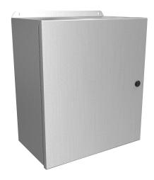
Hammond Eclipse Junior series enclosure, NEMA 3R/4/4X/12/13, 16 x 14 x 8in (HxWxD), wall mount, 5052-H32 aluminum, singledoor, 1/4-turn semi-flush 316 stainless steel latch.
