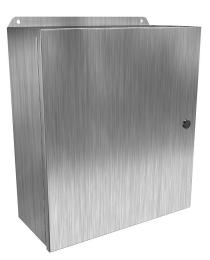
Hammond Eclipse Junior series enclosure, NEMA 3R/4/4X/12/13, 16 x 14 x 6in (HxWxD), wall mount, 304 stainless steel, #4 brush finish, single-door, 1/4-turn semi-flush 316 stainless steel latch.
