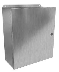
Hammond Eclipse Junior series enclosure, NEMA 3R/4/4X/12/13, 16 x 14 x 6in (HxWxD), wall mount, 316 stainless steel, #4 brush finish, single-door, 1/4-turn semi-flush 316 stainless steel latch.
