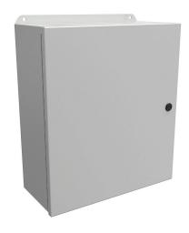
Hammond Eclipse Junior series enclosure, NEMA 3R/4/12/13, 16 x 14 x 6in (HxWxD), wall mount, carbon steel, RAL 7035 light gray, powder coat finish, single-door, 1/4-turn semi-flush latch.
