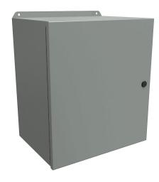
Hammond Eclipse Junior series enclosure, NEMA 3R/4/12/13,  $16 \times 14 \times 10$  in (HxWxD), wall mount, carbon steel, ANSI 61 gray, powder coat finish, single-door, 1/4-turn semi-flush latch.
