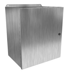
Hammond Eclipse Junior series enclosure, NEMA 3R/4/4X/12/13,  $16 \times 14 \times 10$  in (HxWxD), wall mount, 304 stainless steel, #4 brush finish, single-door, 1/4-turn semi-flush 316 stainless steel latch.
