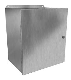
Hammond Eclipse Junior series enclosure, NEMA 3R/4/4X/12/13,  $16 \times 14 \times 10$  in (HxWxD), wall mount, 316 stainless steel, #4 brush finish, single-door, 1/4-turn semi-flush 316 stainless steel latch.
