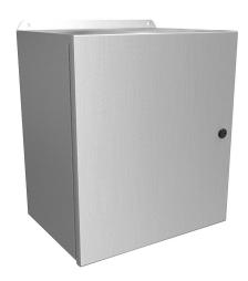
Hammond Eclipse Junior series enclosure, NEMA 3R/4/4X/12/13, 16 x 14 x 10in (HxWxD), wall mount, 5052-H32 aluminum, singledoor, 1/4-turn semi-flush 316 stainless steel latch.
