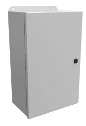
Hammond Eclipse Junior series enclosure, NEMA 3R/4/12/13, 16 x 10 x 6in (HxWxD), wall mount, carbon steel, RAL 7035 light gray, powder coat finish, single-door, 1/4-turn semi-flush latch.
