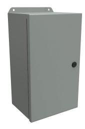
Hammond Eclipse Junior series enclosure, NEMA 3R/4/12/13,  $14 \times 8 \times 6$  in (HxWxD), wall mount, carbon steel, ANSI 61 gray, powder coat finish, single-door, 1/4-turn semi-flush latch.
