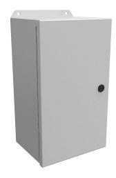
Hammond Eclipse Junior series enclosure, NEMA 3R/4/12/13,  $14 \times 8 \times 6$  in (HxWxD), wall mount, carbon steel, RAL 7035 light gray, powder coat finish, single-door, 1/4-turn semi-flush latch.
