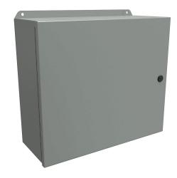
Hammond Eclipse Junior series enclosure, NEMA 3R/4/12/13, 14 x 16 x 6in (HxWxD), wall mount, carbon steel, ANSI 61 gray, powder coat finish, single-door, 1/4-turn semi-flush latch.
