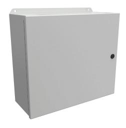
Hammond Eclipse Junior series enclosure, NEMA 3R/4/12/13, 14 x 16 x 6in (HxWxD), wall mount, carbon steel, RAL 7035 light gray, powder coat finish, single-door, 1/4-turn semi-flush latch.
