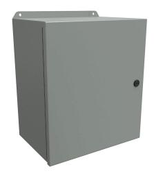
Hammond Eclipse Junior series enclosure, NEMA 3R/4/12/13, 14 x 12 x 8in (HxWxD), wall mount, carbon steel, ANSI 61 gray, powder coat finish, single-door, 1/4-turn semi-flush latch.
