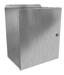
Hammond Eclipse Junior series enclosure, NEMA 3R/4/4X/12/13,  $14 \times 12 \times 8$  in (HxWxD), wall mount, 316 stainless steel, #4 brush finish, single-door, 1/4-turn semi-flush 316 stainless steel latch.
