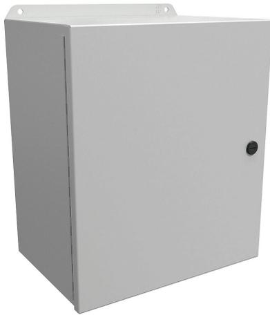
Hammond Eclipse Junior series enclosure, NEMA 3R/4/12/13, 14 x 12 x 8in (HxWxD), wall mount, carbon steel, RAL 7035 light gray, powder coat finish, single-door, 1/4-turn semi-flush latch.
