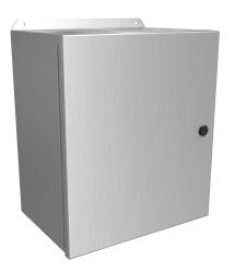
Hammond Eclipse Junior series enclosure, NEMA 3R/4/4X/12/13, 14 x 12 x 8in (HxWxD), wall mount, 5052-H32 aluminum, single-door, 1/4-turn semi-flush 316 stainless steel latch.
