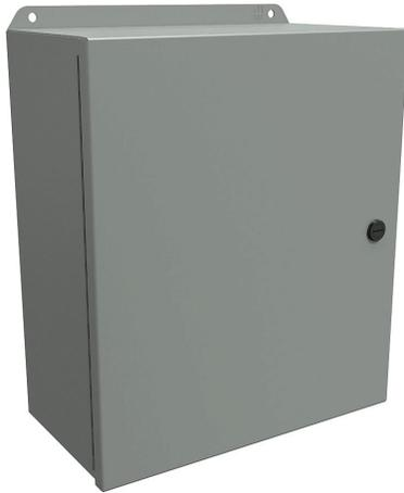
Hammond Eclipse Junior series enclosure, NEMA 3R/4/12/13, 14 x 12 x 6in (HxWxD), wall mount, carbon steel, ANSI 61 gray, powder coat finish, single-door, 1/4-turn semi-flush latch.
