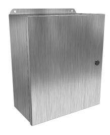
Hammond Eclipse Junior series enclosure, NEMA 3R/4/4X/12/13,  $14 \times 12 \times 6$  in (HxWxD), wall mount, 304 stainless steel, #4 brush finish, single-door, 1/4-turn semi-flush 316 stainless steel latch.
