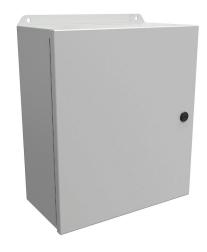
Hammond Eclipse Junior series enclosure, NEMA 3R/4/12/13, 14 x 12 x 6in (HxWxD), wall mount, carbon steel, RAL 7035 light gray, powder coat finish, single-door, 1/4-turn semi-flush latch.
