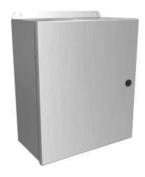
Hammond Eclipse Junior series enclosure, NEMA 3R/4/4X/12/13, 14 x 12 x 6in (HxWxD), wall mount, 5052-H32 aluminum, singledoor, 1/4-turn semi-flush 316 stainless steel latch.
