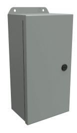
Hammond Eclipse Junior series enclosure, NEMA 3R/4/12/13,  $12 \times 6 \times 4$ in (HxWxD), wall mount, carbon steel, ANSI 61 gray, powder coat finish, single-door, 1/4-turn semi-flush latch.
