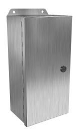
Hammond Eclipse Junior series enclosure, NEMA 3R/4/4X/12/13, 12 x 6 x 4in (HxWxD), wall mount, 304 stainless steel, #4 brush finish, single-door, 1/4-turn semi-flush 316 stainless steel latch.
