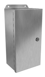
Hammond Eclipse Junior series enclosure, NEMA 3R/4/4X/12/13, 12 x 6 x 4in (HxWxD), wall mount, 316 stainless steel, #4 brush finish, single-door, 1/4-turn semi-flush 316 stainless steel latch.
