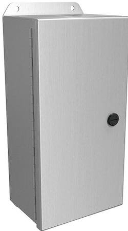
Hammond Eclipse Junior series enclosure, NEMA 3R/4/4X/12/13, 12 x 6 x 4in (HxWxD), wall mount, 5052-H32 aluminum, single-door, 1/4-turn semi-flush 316 stainless steel latch.
