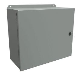
Hammond Eclipse Junior series enclosure, NEMA 3R/4/12/13, 12 x 14 x 6in (HxWxD), wall mount, carbon steel, ANSI 61 gray, powder coat finish, single-door, 1/4-turn semi-flush latch.
