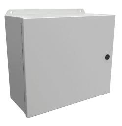
Hammond Eclipse Junior series enclosure, NEMA 3R/4/12/13, 12 x 14 x 6in (HxWxD), wall mount, carbon steel, RAL 7035 light gray, powder coat finish, single-door, 1/4-turn semi-flush latch.
