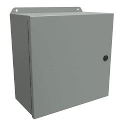
Hammond Eclipse Junior series enclosure, NEMA 3R/4/12/13, 12 x 12 x 6in (HxWxD), wall mount, carbon steel, ANSI 61 gray, powder coat finish, single-door, 1/4-turn semi-flush latch.
