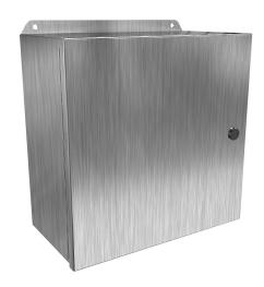
Hammond Eclipse Junior series enclosure, NEMA 3R/4/4X/12/13,  $12 \times 12 \times 6$  in (HxWxD), wall mount, 304 stainless steel, #4 brush finish, single-door, 1/4-turn semi-flush 316 stainless steel latch.
